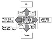
To use this four-way key, place your thumb over the key on the handset and move to the four positions to get the feel of how it moves and operates.
